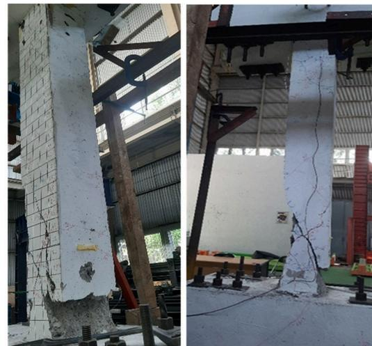
Figure 16. Damage pattern in the first step
